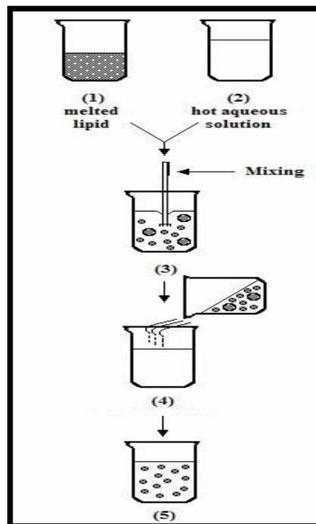
**Figure 4:** Schematic representation of the production of lipid nanoparticles via microemulsions.
