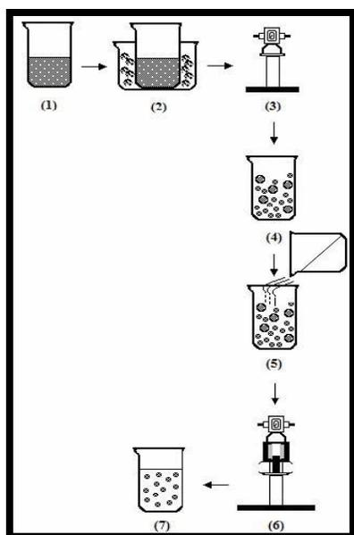
**Figure 3:** Schematic representation of the production of lipid nanoparticles by cold HPH method.
