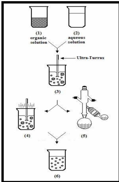
**Figure 5:** Schematic representation of the production of lipid nanoparticles by solvent emulsification-evaporation method.
