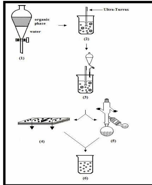
**Figure 6:** Schematic representation of the production of lipid nanoparticles by emulsification-diffusion method.
