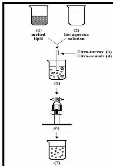
**Figure 2:** Schematic representation of the production of lipid nanoparticles by hot HPH method.
