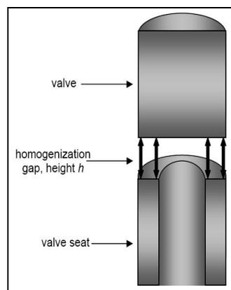
**Figure 1:** The geometry of the homogenization valve (valve and valve seat) and the resulted homogenization gap between them.
