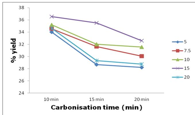
**Figure 3:** Effect of carbonization time on yield of activated carbon (H<sub>3</sub>PO<sub>4</sub>) at 500°C
