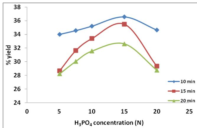
**Figure 1:** Effect of  $H_3PO_4$  concentration on yield of activated carbon at 500°C.
