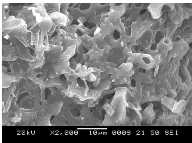
**Figure 4:** SEM images of activated carbon
