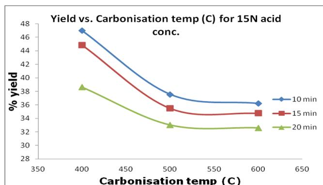
**Figure 2:** Effect of carbonization temperature on yield of activated carbon (15 N  $H_3PO_4$ )
